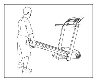
2. Hold the treadmill firmly with your left hand. Using your right hand, pull the latch knob to the right and hold it. Raise the treadmill until the pin on the latch knob is aligned with the hole in the left foam grip. Then, release the latch knob. Make sure that the latch knob is fully released so that the pin is fully inserted into the hole in the left foam grip.
